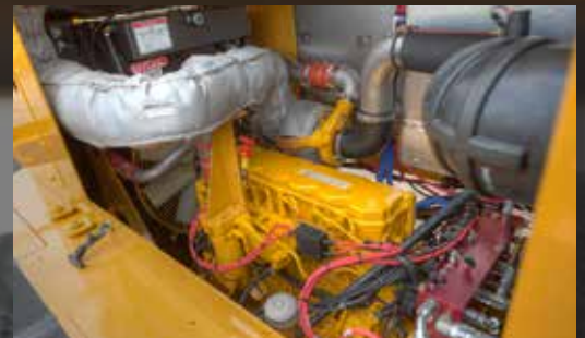
QSB-6.7 Liter Cummins Electronic Turbocharged Diesel Engine
