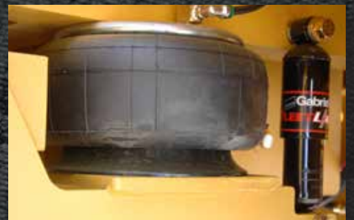
Goodyear® air springs, stabilizing shock absorbers, and isolation mounts
