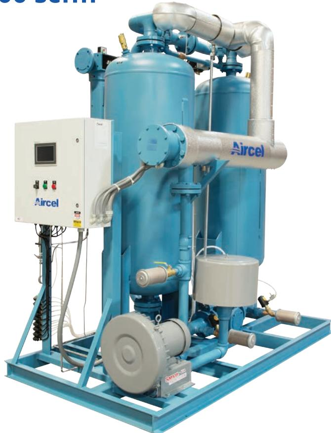
The ABP Series was created with energy savings and efficient usability in mind. A high efficiency blower brings in ambient air for the regeneration cycle while the Energy Management System and unique Parallel Cooling Mode work seamlessly to create maximum energy savings to the bottom line.
