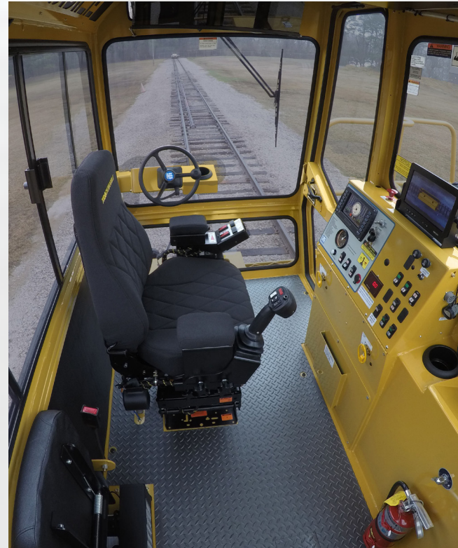
Viking control panel and operational controls.
