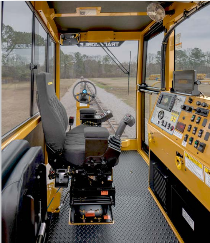
Titan control panel and operational controls.
