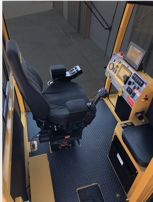
Spartan control panel and operational controls.
