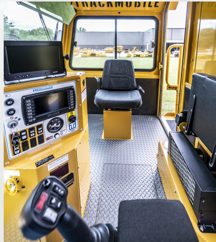
Hercules control panel and operational controls.
